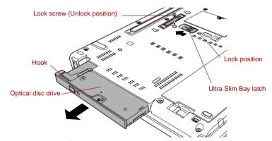
Figure 4-19 Removing the optical disc drive
